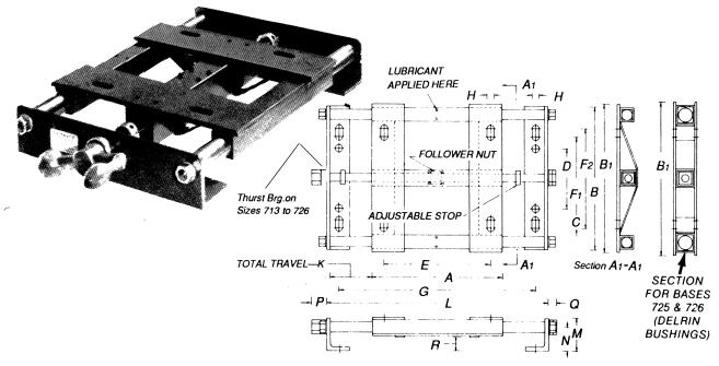
The 700 Series is for use with motors equipped with spring loaded variable-pitch pulleys on which one or both flanges are movable and where the driven pulley is grooved or has a standard flat. Where one flange is movable, the driven pulley should have a wide flat—not crowned. Use the 800 Series with pulleys with one flange movable with either a standard or grooved driven pulley.
